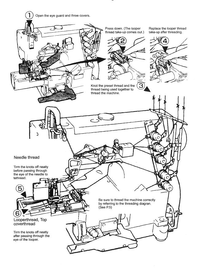
Threading diagram (2-needle, 3-needle)
